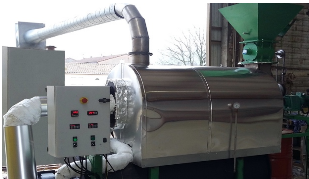
CarboChar-1 is the most compact model. It can produce up to 1 tonne of green charcoal per day. The larger model, CarboChar-3, can produce up to 5 tonnes per day.
